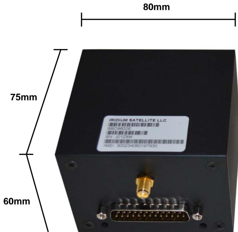
Figure 1 - Dimensions of housing
