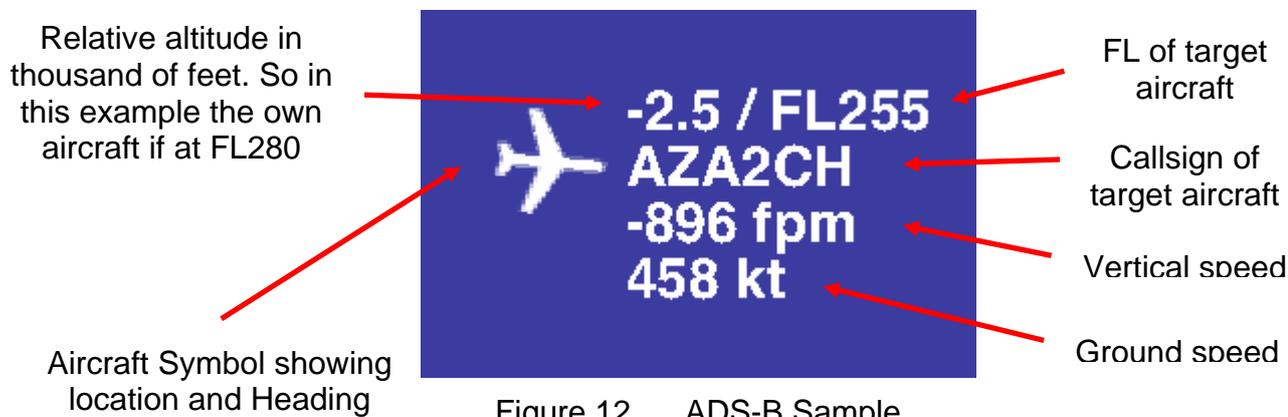
Please note if the own aircraft is broadcasting ADS-B and the proper callsign for the own ship has been set on the config page, the relative altitude will be calculated based on the reported baro altitude. If this data is not available GPS altitude will be used which can be several hundred feet off depending on atmospheric conditions.
