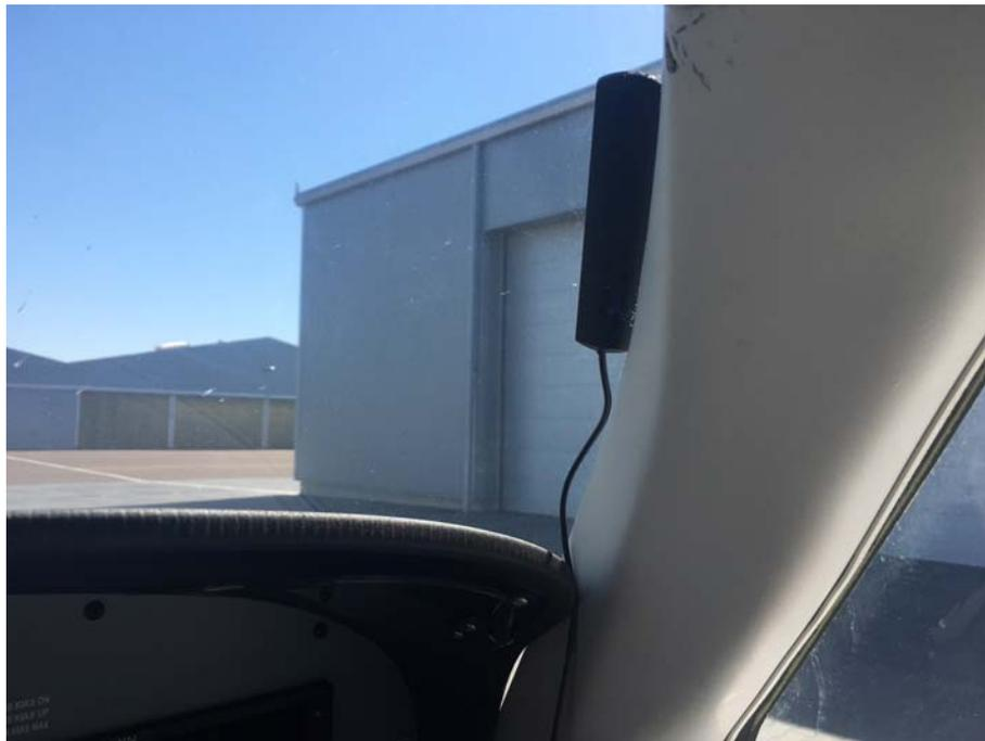
Figure 4 ADS-B Antenna Example
