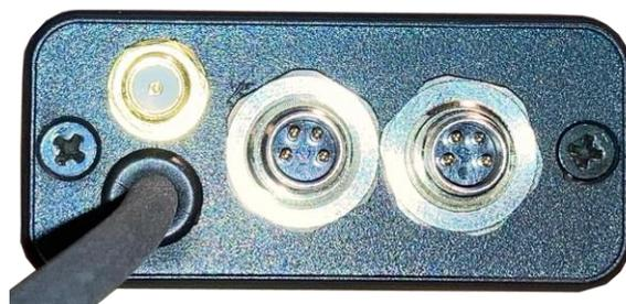
Figure 2 ADLS1G front with SMA connector (left) Port 2 (middle) and Port (right)
