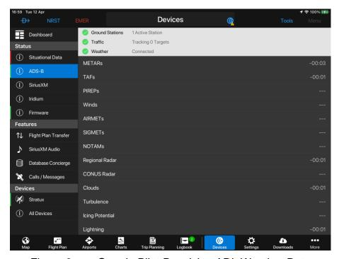
Figure 9 Garmin Pilot Receiving ADL Weather Data
