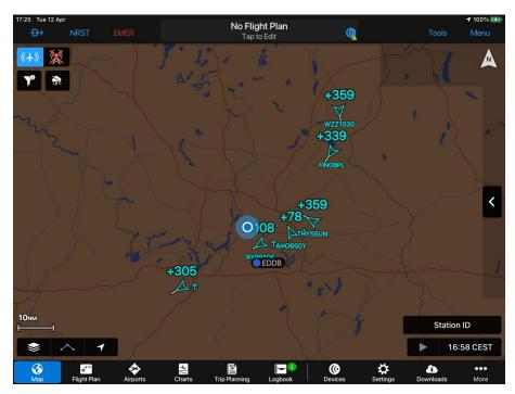
Figure 14 Garmin Pilot Showing ADL Traffic
