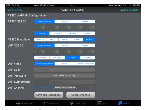
Figure 6 WiFi GDL90 Configuration for Devices ADL140 and later
